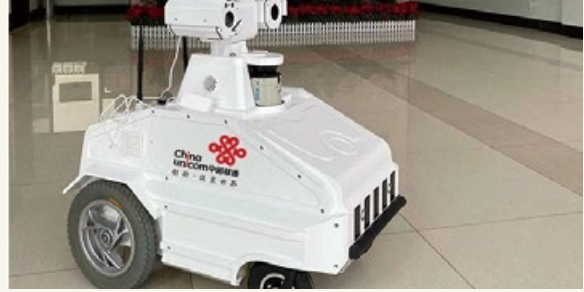
Patrol robot equipped with 5G+ infrared body temperature detection
